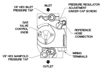
Figure 43 – Combination Gas Valve
